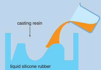
Pour the casting resin into the silicone rubber mold and let it cure. You can lengthen the life of the silicone rubber mold if you apply a releasing agent as necessary.
