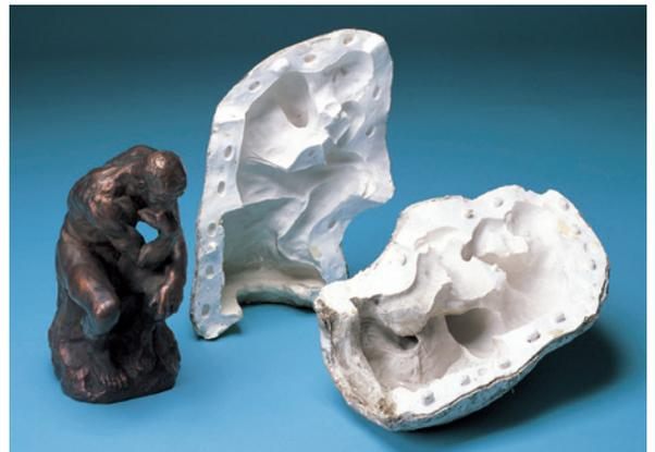
Casting of low-melting-point alloy
