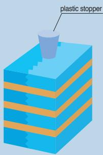
Assemble the mold, place boards on both sides and fix them securely into place using rubber rings and clamps and place a plastic stopper in the gate.
