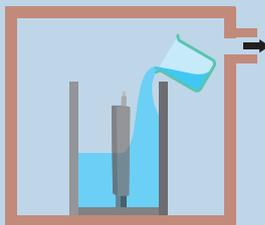
Under depressurized conditions, pour in liquid silicone rubber until the master is completely covered.
