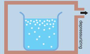
Extract remaining trapped air with a vacuum chamber.
