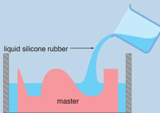
Pour in the liquid silicone rubber until the master is completely covered and carry out secondary de-airing to eliminate all bubbles from the liquid silicone rubber. If you do not have a vacuum chamber, use a brush to spread the liquid silicone rubber uniformly over the surface of the master first until all air pockets on the surface have been removed and then pour in the rest of the liquid silicone rubber.
