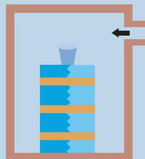
Once atmospheric pressure has been restored, the resin will flow into the mold. Cure the resin under the specified conditions (temperature and humidity).
