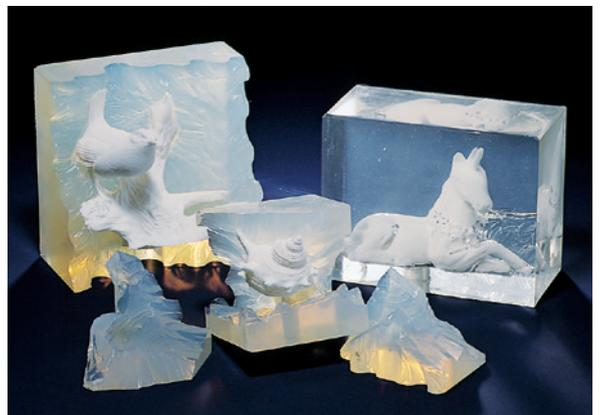
Transparent and translucent liquid silicone rubber moldmaking
