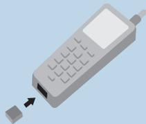
Affix the gate, which serves as the opening for pouring in the casting resin, to the master.
