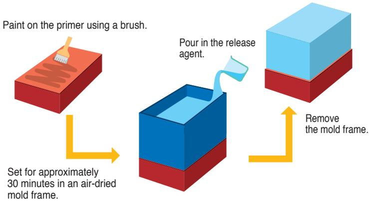
Table 5 Primer for two-component liquid silicone rubber
