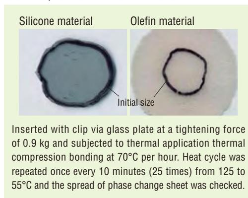
Inserted with clip via glass plate at a tightening force of 0.9 kg and subjected to thermal application thermal compression bonding at 70°C per hour. Heat cycle was repeated once every 10 minutes (25 times) from 125 to 55°C and the spread of phase change sheet was checked.
