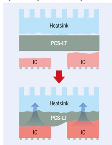
Photo3: Pump out in silicone versus olefin materials
