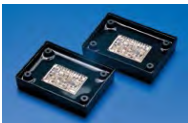
Electronic components potted with silicone gel
