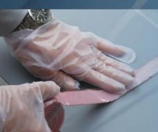
Cat-tape cures and bonds in 24 hours after application, and bonds strongly to both Catpad sheets and mortar foundation surfaces.
