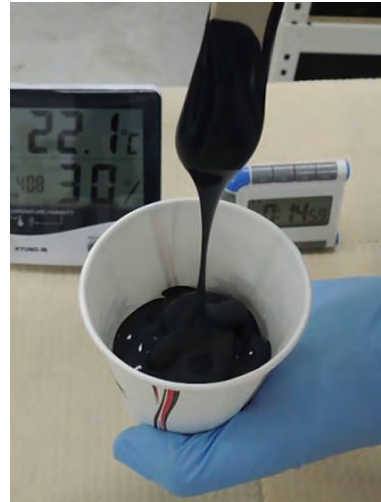
Uncured (The sealant doesn't reach snap time)
