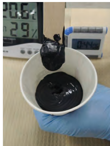
Uncured (The sealant reached snap time)
