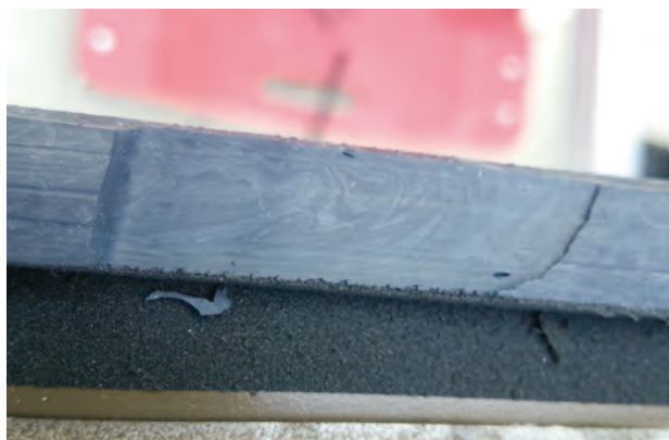
NG Mode (Insufficient mixing)
