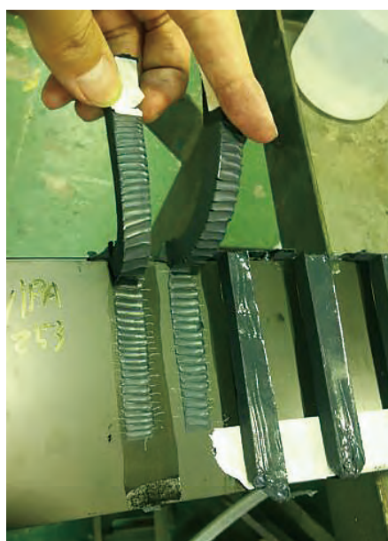
OK Mode (Cohesive failure)
