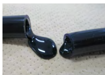
30 minutes after potting Consistency: Liquid
