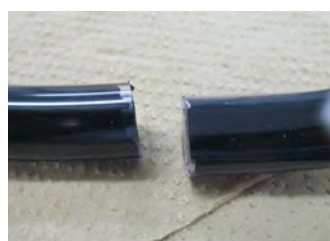
3-5 hours after potting Consistency: Rubber elastic body
