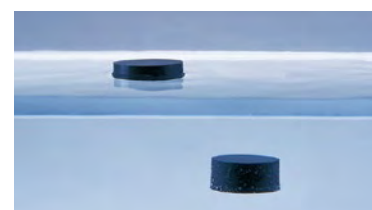
Low-density silicone rubber molded product floating on water
