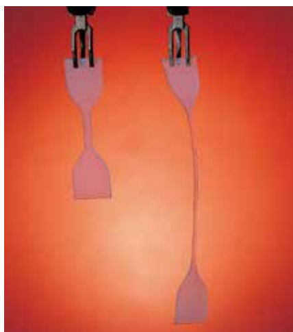
Crosslinked polyethylene: heat resistance test
