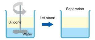
Mixing silicone and water together with a surfactant
