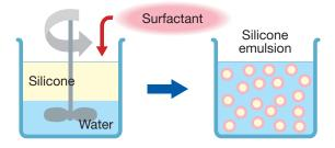
The size of the micelles is typically referred to as the emulsion particle size. For most silicone emulsions, this is between 0.2  $\mu$ m and 0.5  $\mu$ m.
