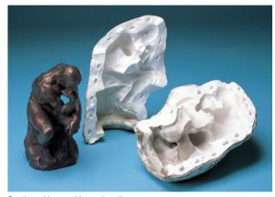
Casting of low-melting-point alloy
