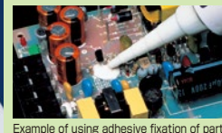
Example of using adhesive fixation of parts
