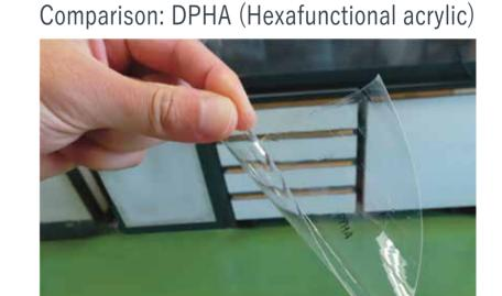
A composition containing 2 wt% of a photoinitiator is applied to a PET film and cured at 600 mJ/cm² under N2 atmosphere.
